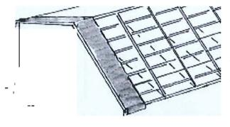
Starting at the end of the roofing framework, measure the length across the trusses, adding enough to allow overhang at both ends. Cut the first piece and lay in place. Pull tight from both ends and attach to trusses or purlins using selftapping screws and washers or with pressuresensitive reflective tape. Cut the second length, laying parallel to first. Make sure to butt or slightly overlap edges. Tape all seams.
